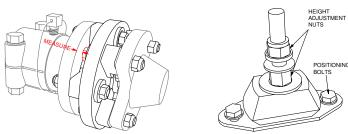
ENGINE MOUNT POSITIONING BOLTS AND HEIGHT ADJUSTMENT NUTS MAY WORK LOOSE RESULTING IN MISALIGNMENT.
