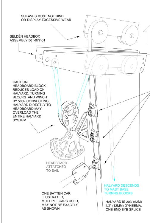
SEE THE SELDÉN MANUAL FOR REGULAR SERVICE TO THE MAST HEADBOX SHEAVES WHICH CAN BE SERVICED WITHOUT LOWERING SPAR OR UNREAVING HALYARDS BY LIFTING OUT THE DIVIDER PLATE AND SHEAVE ASSEMBLIES
