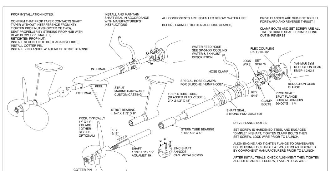
SHAFT BEARINGS ARE "CUTLESS" TYPE AND ARE LINED WITH FLUTED RUBBER. CLEARANCE IS LARGE AND MAY BE UP TO .075" BEFORE RENEWAL. FISHING LINE WRAPS WILL DAMAGE RUBBER INSERT, ROPE WRAPS MAY DAMAGE BEARING AND TUBE ASSEMBLY
