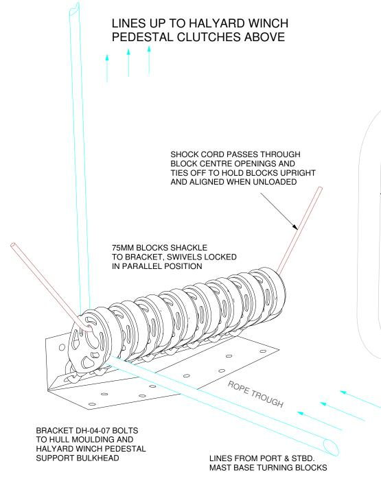
HARKEN RECOMMENDS THAT THE BLOCKS BE FREQUENTLY FLUSHED WITH FRESH WATER TO REMOVE SALT DEPOSITS AND DIRT.
