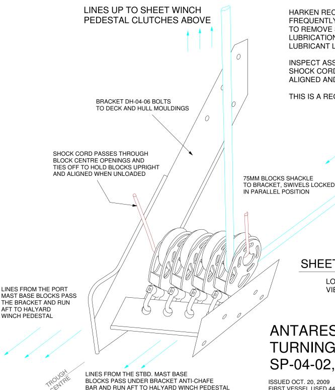
HARKEN RECOMMENDS THAT THE BLOCKS BE FREQUENTLY FLUSHED WITH FRESH WATER TO REMOVE SALT DEPOSITS AND DIRT. LUBRICATION WITH A NON-DIRT ATTRACTING LUBRICANT LIKE HARKEN McLUBE MAY BE APPLIED.
