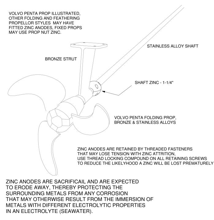
THE ZINC LONGEVITY WILL VARY ACCORDING TO THE QUANTITY OF PROTECTED METAL AND THE ENVIRONMENTAL CONDITIONS INCLUDING; WATER TEMPERATURE, SALINITY, POLLUTANTS, NEARBY METALLIC OBJECTS AND NEIGHBOURING BOAT OR SHORE ELECTRICAL INSTALLATIONS.
